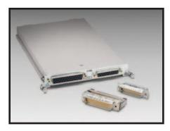
The Model 7709 plug-in module is a two-pole, 6×8 matrix module. It can connect any combination of six differential channels of instrumentation to any combination of eight differential device-under-test channels. The instrumentation can be AC and DC sources, internal or external meters, oscilloscopes, etc. This matrix configuration allows wide flexibility for complex test systems.
